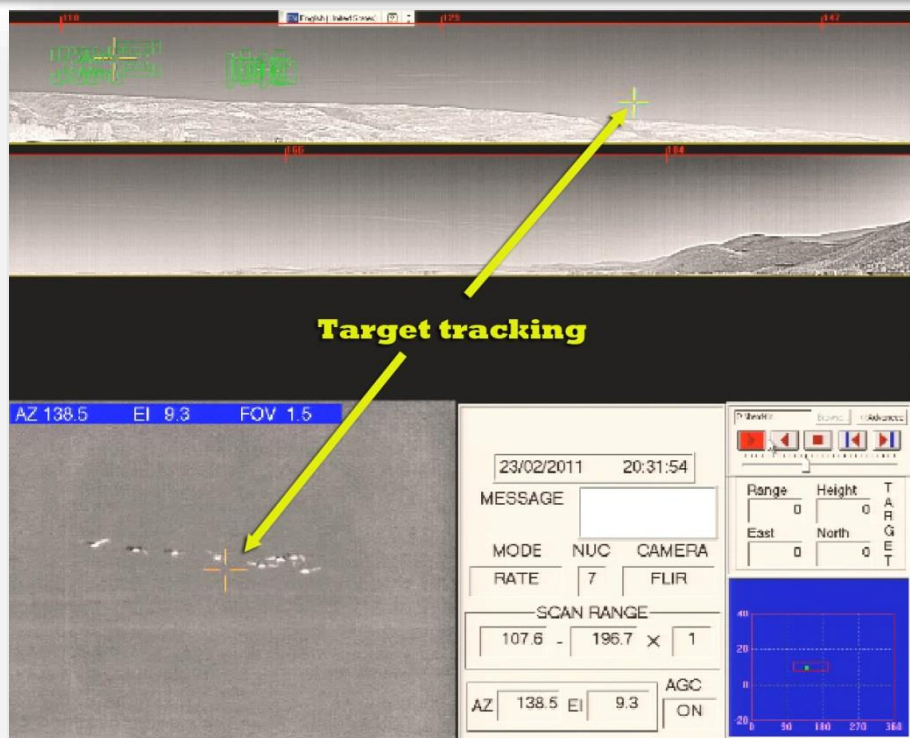
Figure 16: INTERCEPTOR infrared tracking system. Once a target group of birds is marked by the user in the panoramic display, the system automatically tracks the birds as they move through the environment. Zoom capabilities are simultaneously operational while in tracking mode.
