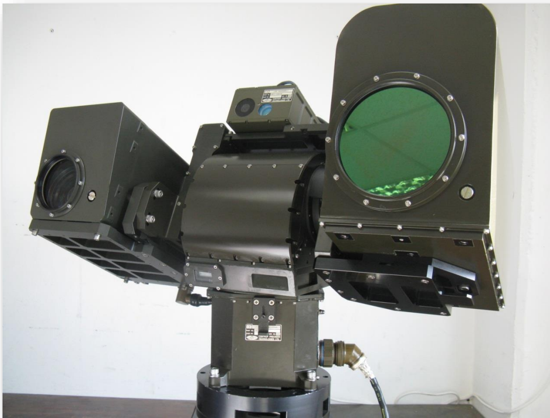
Figure 1: INTERCEPTOR System Payload. IR camera is located on the right-hand side of the system. CCD camera on the left-hand side. Long-range laser range finder is located on the top portion of the unit. All components are separately removable and customizable.
