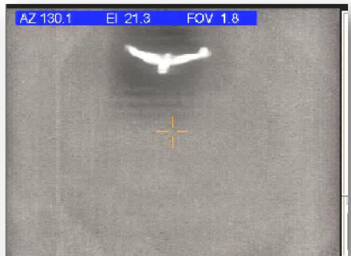
Figure 12: FLIR detector closeup of hawk at 15x zoom at a range of approximately 7 km.
